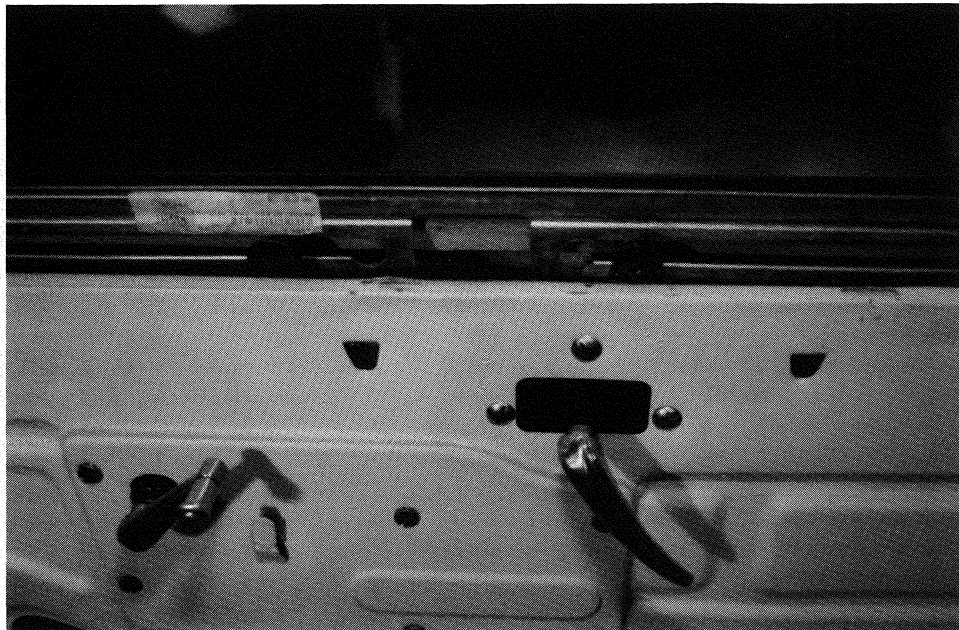
Figure (18) Window channel engaged with regulator
