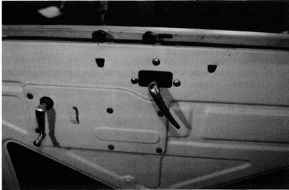
Figure (17) Window regulator installed with arm and buttons positioned for engagement with metal window channel
