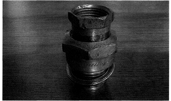
The modified base of a 3X spark plug and the adapter attached with 1/2"-20 threads.
