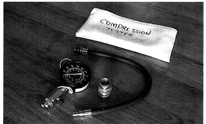
Everything that is needed to run a compression test while standing along side the road.
