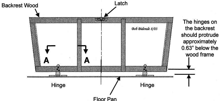
The backrest frame is centered between the floor pan hinges. See View A-A for the vertical position of the backrest hinges, and variations in the position of the hinges reported by some Association members.
